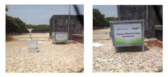
Photograph 9: Noise Monitoring station at Runway path carrying out continues noise monitoring at MIAL.
